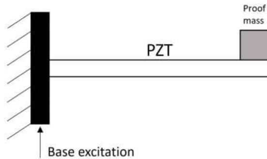
Figure 8. Basic cantilever based PEH configuration
